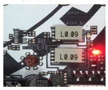
However, if the active BIOS\_A1 is corrupted or damaged, after several failed boot attempts, it will automatically do BIOS recovery from the backup BIOS\_B1 and then the system will still work on the active BIOS\_A1. And the monitor will show Secure Backup UEFI (B-->A) function as picture below.
