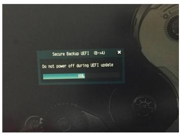
After finishing this function, the system will reboot and work on the active BIOS\_A1.
